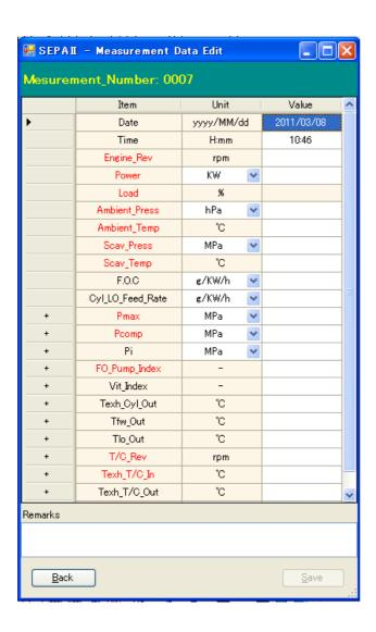
Only the same input data as main engine performance data sheet is required for the engine performance analysis.
