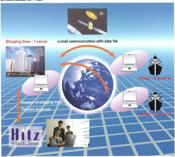
The capacity of 1 performance data is limited about to 1 KB. By communication with only 1 KB data file, at anywhere of the vessel, the shipping company and Hitachi Zosen, the same graphs and images can be shared to monitor.
